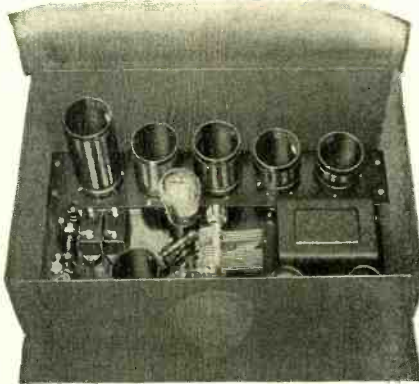
National Thrill Box, 4-tube short wave circuit, 15 to 535 meters, battery-operation of filaments; B supply, either batteries or eliminator.
